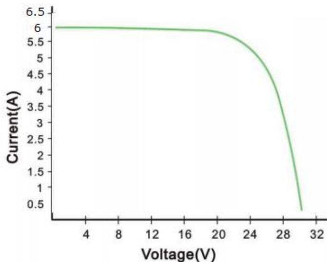
Note: All electrical parameters are rated at standard test conditions (irradiance of 1000W/m<sup>2</sup>, AM 1.5G, cell temperature 77F/25°C)
